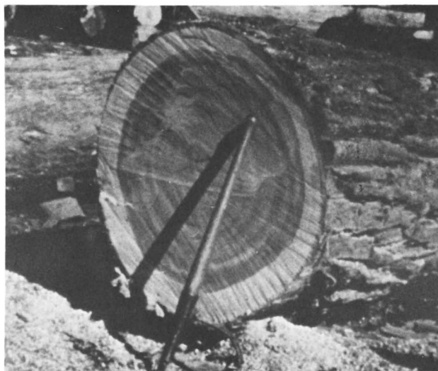
Figure 1. End view of a log showing both the wood and bark. Note the small total volume occupied by the bark. The central, dark portion of the wood is heartwood, and the outer ring of light colored wood is sapwood.
